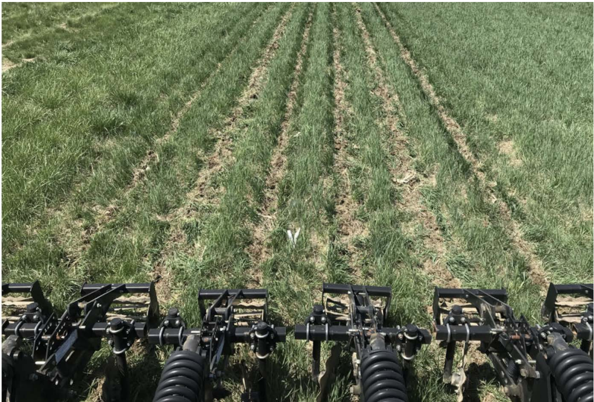
Figure 1. Kernza IWG field after the mechanical thinning practice of strip-tillage using a Unverferth Zone Builder Subsoiler Model 122. Image from Law et al., 2020.
