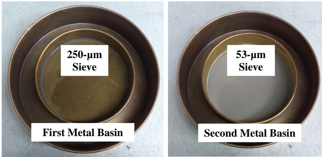
Figure A.2 Microaggregate isolator used in Step B of aggregate fractionation.
