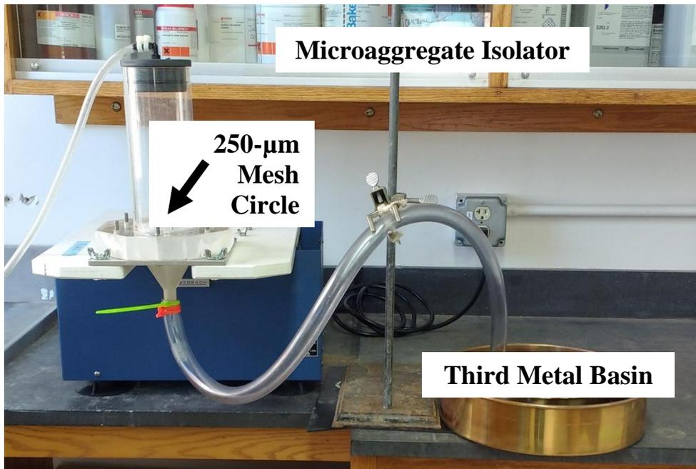
Figure A.3 250- $\mu\text{m}$  mesh circle and final sieve and metal basin used in microaggregate isolation (Step B) of aggregate fractionation.
